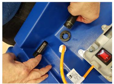
2. Unscrew the grey cable gland to free up the orange electricity cable from the tank. Remove the other side of the cable from the switch located in the battery holder (4 screws to remove the battery holder), pass cable throught the cable cable into the tank.
