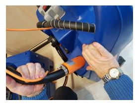
1. Remove the hose and the electricity cable from the trolley in order to take the pump out and replace it
