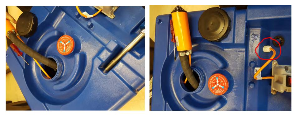
4. Now you can connect the new electricity cable to the battery switch.
